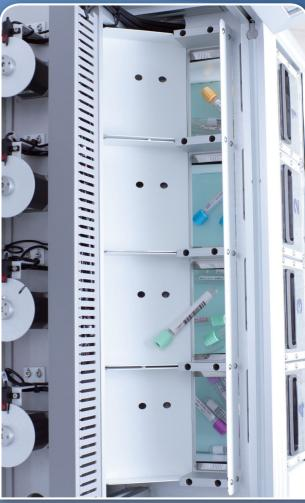
Sort out sample tubes to a specified bin through barcode information. (8 bins)
