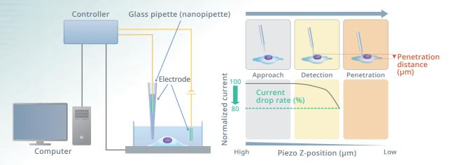
\*A scanning Ion Conductance Microscope: acquires the surface 3D shape of a material by utilizing the decrease in ion current value that occurs as the distance between the probe (glass pipette) and the sample (cells, etc.) gets closer. The SU10 does not have an image acquisition function
