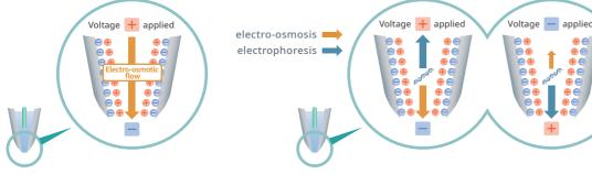
Since the inner wall of the nanopipette is negatively charged, cations and other ions in the liquid inside the nanopipette form an ionic layer. The ionic layer moves toward the tip of the nanopipette when a higher voltage is applied than at the time of approach. The movement of the ionic layer causes the liquid in the nanopipette to move (electro-osmotic flow) and is injected into the cell.
