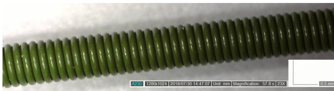
Spring coils made with T-Glide wire - strong coating adhesion and scratch resistance observed.
